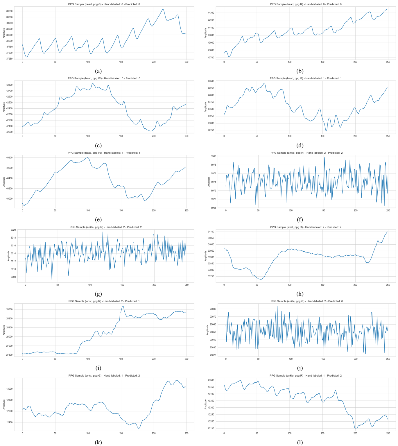
Figure 8: Example PPG Traces: (a)-(b): Correctly identified as good quality traces. (c): Trace with baseline drift that can be filtered away, as the pulse shape remains clearly visible. (d): Classified as "fair" due to some noise and intermediate pulses. (e): Traces containing baseline drift that affects peak height and is difficult to filter away. (f)-(g): Pure noise correctly identified as poor quality. (h): Up and down movement too wide for a pulse, correctly classified as poor. (i): Up and down movement without recognizable pulses, but the algorithm incorrectly identifies some pulses, classifying it as fair. (j): Noisy signal misclassified as good by the algorithm. (k)-(l): When correlated with ECG, pulses can be recognized (would be fair quality), but the algorithm incorrectly rejects these as poor.
